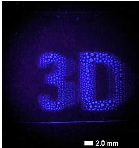
Figure 38: "3D" printed with polymer solution containing fluorescent ink
