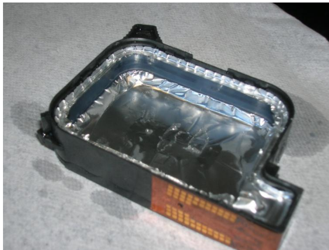
Figure 14: Inside of the cartridge with metal plates and spring removed
