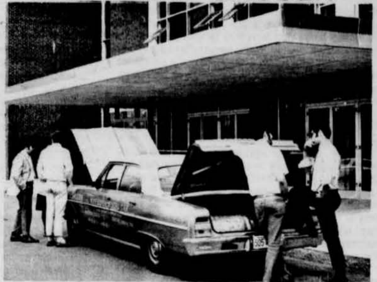
The "Natural Gasser" is a converted 1965 Chevelle powered by bottled propane. Propane costs one-fifth as much as gasoline.
