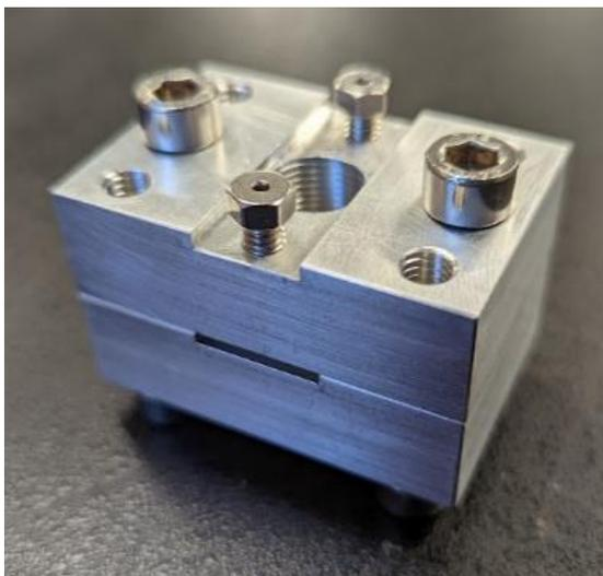
**Figure 14:** Final fabricated reactor chuck
