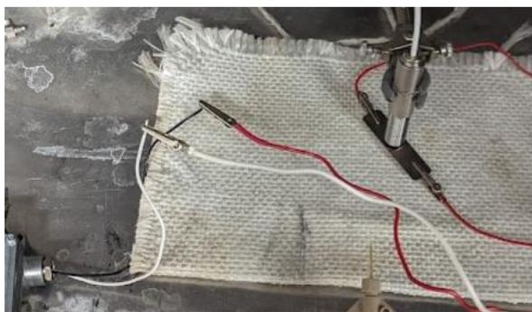
**Figure 9:** Experimental setup for temperature control tests. Includes steel strip connected to power supply with pyrometer and sense leads connected to pyrometer output.
