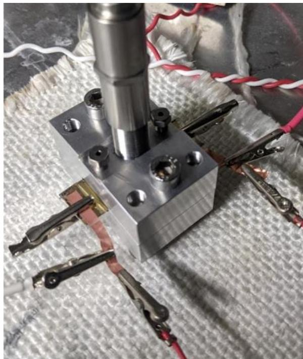
**Figure 8:** *Experimental setup for proof of theory heat tests. Includes reactor, power supply lead, and sense lead configuration.*
