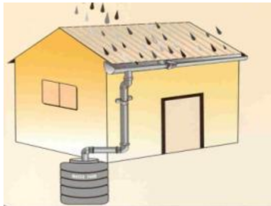
Figure 4: Rooftop rainwater harvesting illustration
