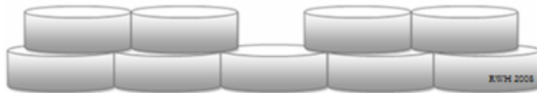
Figure 18: Example of a two-layer tire spillway
