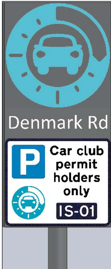
Figure I5 - Bay Location Sign Front
