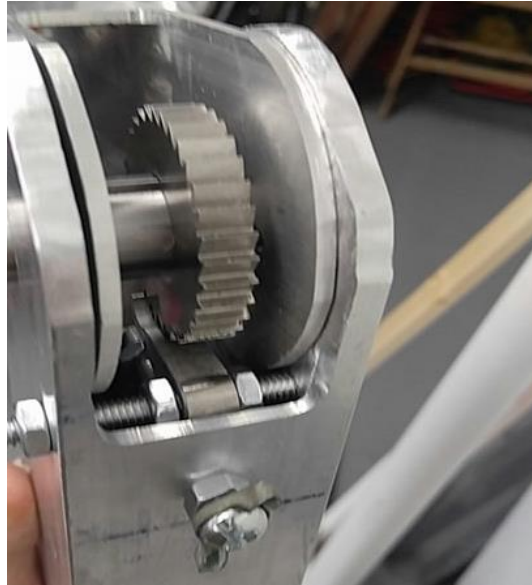
Figure 58: Assembly for the Ratchet Mechanism, Pawl Included
