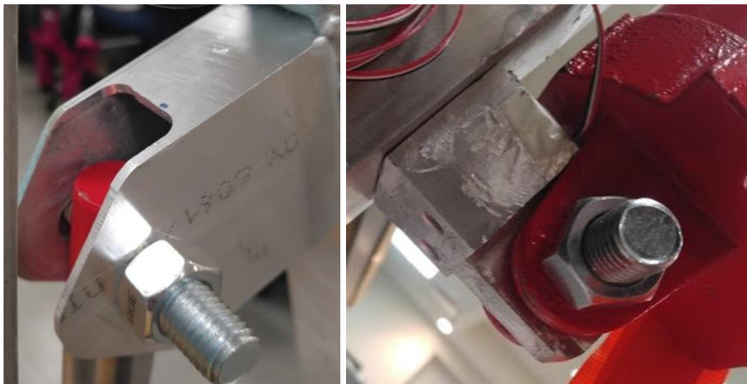
Figure 60: Hydraulic Pump Supports
