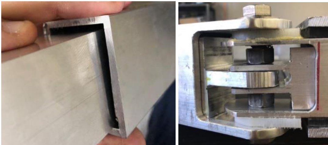
Figure 56: Assembly between the Train- Leg Slider and the Leg Base-Leg Back
