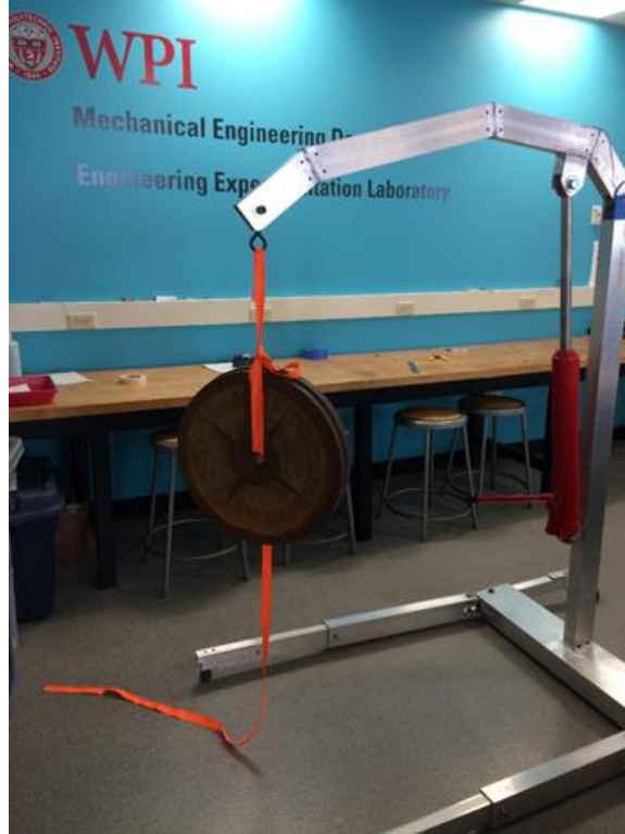
Figure 69: Medical Lifting Prototype Lifting 100 lbs.
