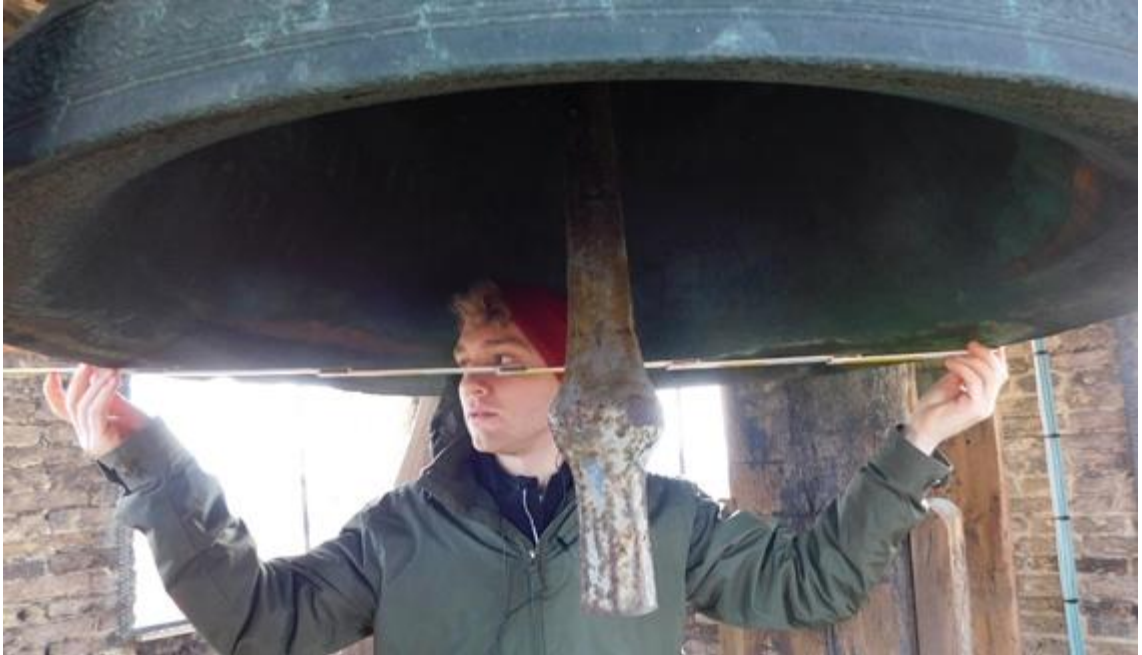
Figure 27 - Measuring the bell diameter
