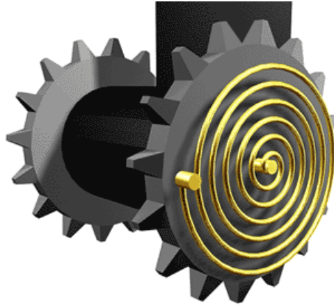
Figure 34: Seatbelt Gear Spring (Harris, 2008)
