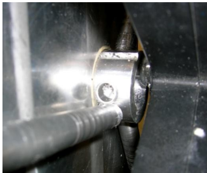
Figure 114: Spoke Stress Failure
