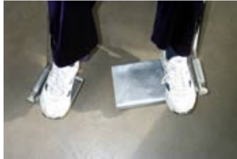
Figure 38: Foot Steering, Cambridge Design Chair (University of Cambridge, 2008)
