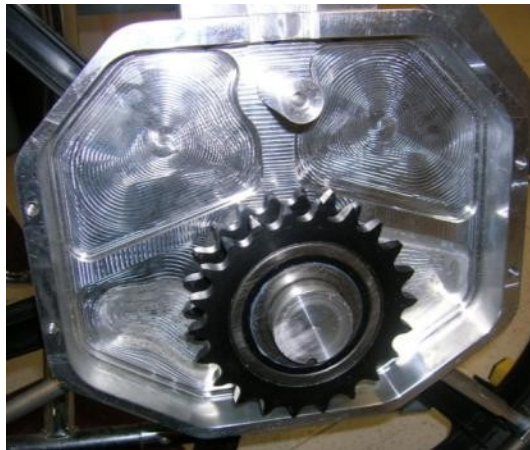
Figure 105: Propulsion System (Backplate, Toothed Wheels, & Clutches)
