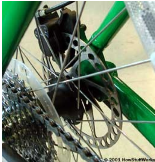
Figure 24: Bicycle Disc Brake (Nice, “How Mountain Bikes Work”, 2008)
