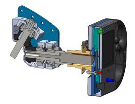
result in less than 1° of backlash in the gearbox. A custom steering wheel was also developed with a multitude of switches, LEDs, and a display to show driving data and facilitate tuning decisions.
