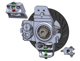
steering load. Both the front and rear uprights utilize camber blocks. They are placed on the upper mounting point and allow for tuning of camber in +/- .5° increments by replacing them with a different block.
