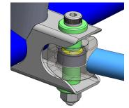
We chose an in-plane pushrod configuration for the dampers and rockers. The resulting in-plane forces allowed for the use of lightweight rockers. Bronze bushings at the pivots allow for smooth
