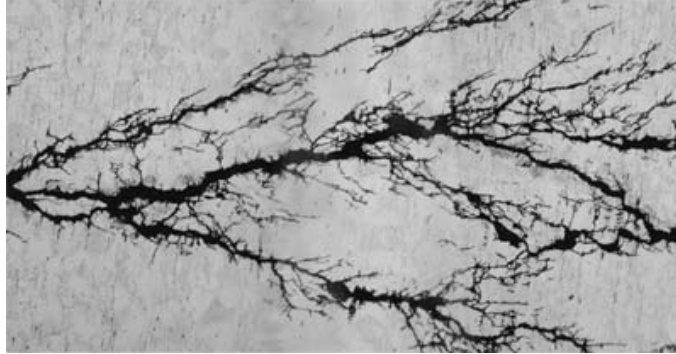
Figure 6: Stress corrosion branching. 15
