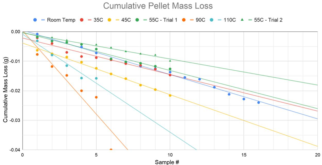
Figure 13: Cumulative pellet mass loss at a range of temperatures
