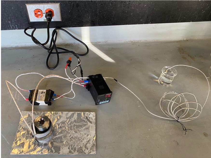
Figure 6: Band heater connected to appropriate controllers
