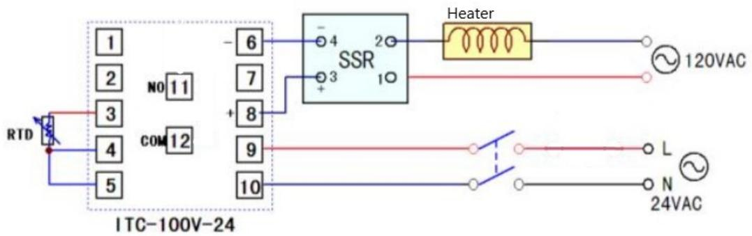
Figure 10:ITC-100VH Wiring diagram
