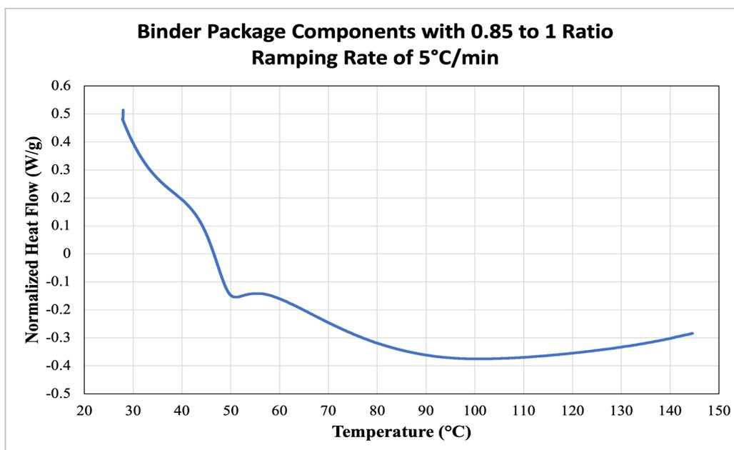
Figure 14: DSC curve at 5°C/min with a PVA to PEG ratio of 0.85:1
