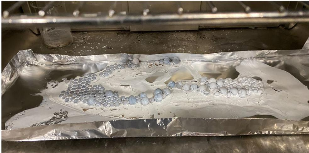
Figure 3: RTP powder pan drying with balls from ball milling
