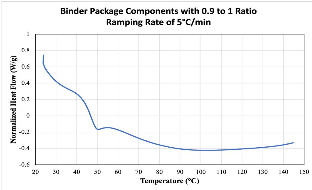
Figure 15: DSC curve at 5°C/min with a PVA to PEG ratio of 0.90:1
