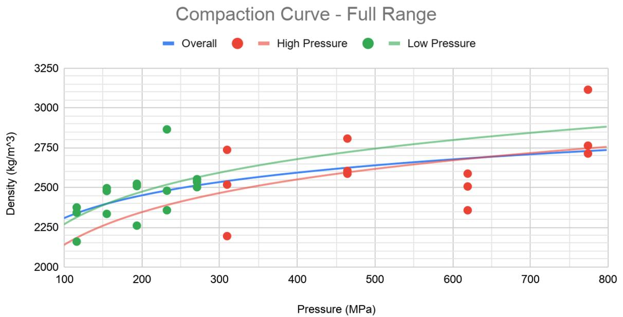
Figure 9: Full Pressure Range vs Density Compaction Curve
