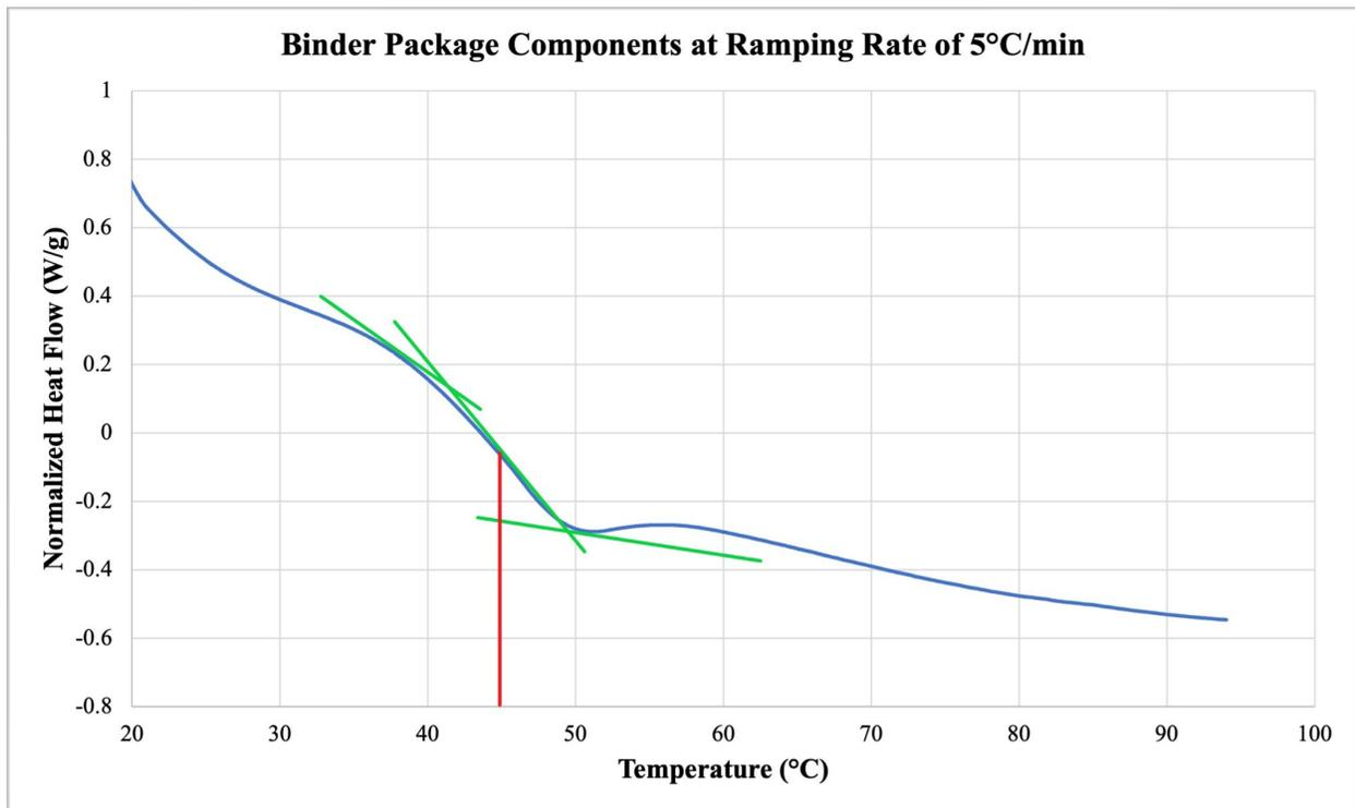
Figure 11: DSC curve at 5°C/min ramping rate with  $T_g$  identified
