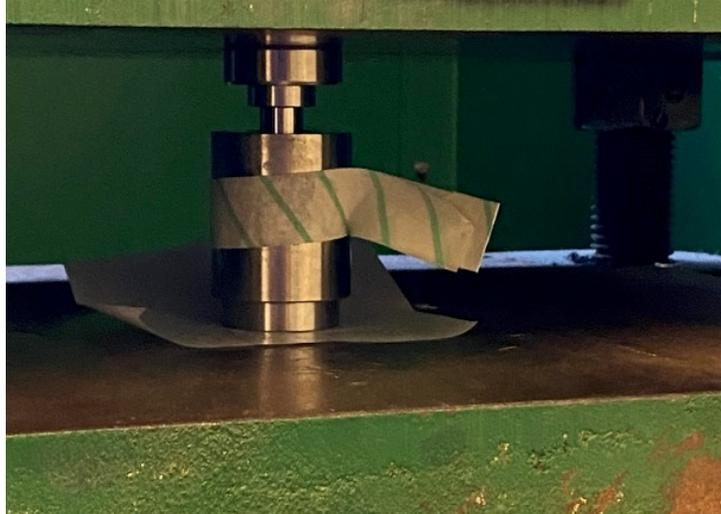
Figure 5: Die under pressure in the press
