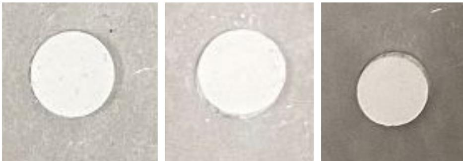
Figure 10: Defect free pellets from lower pressure pressings
