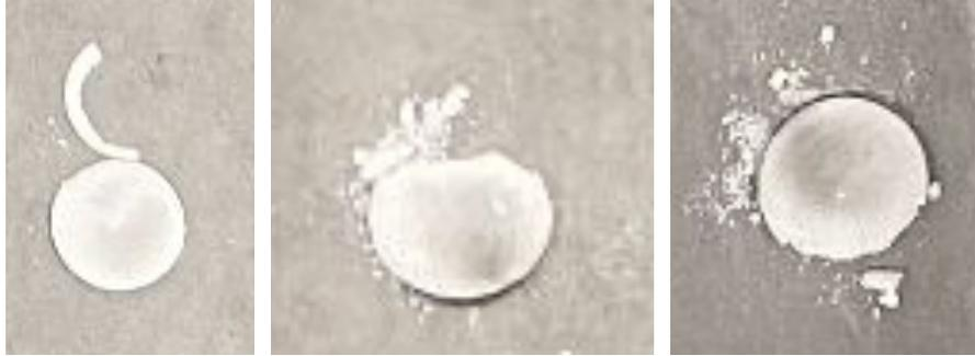
Figure 8: Chipping and uncompressed powder in pellets
