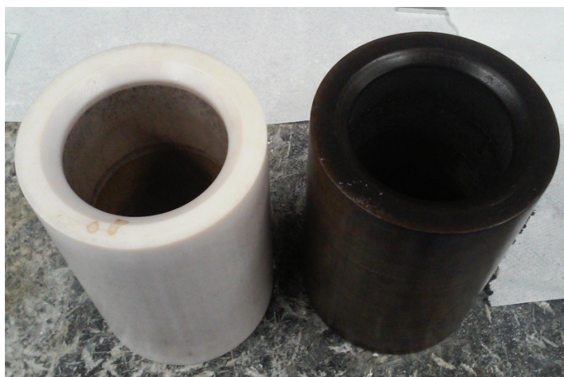
Figure 55. Teflon autoclaves used during hydrochar prep. The autoclave on the right was used for the vast majority of the hydrochar preps. 3-hour, 20-hour, and 72-hour synthesis time hydrochars were prepared using the autoclave on the left.
