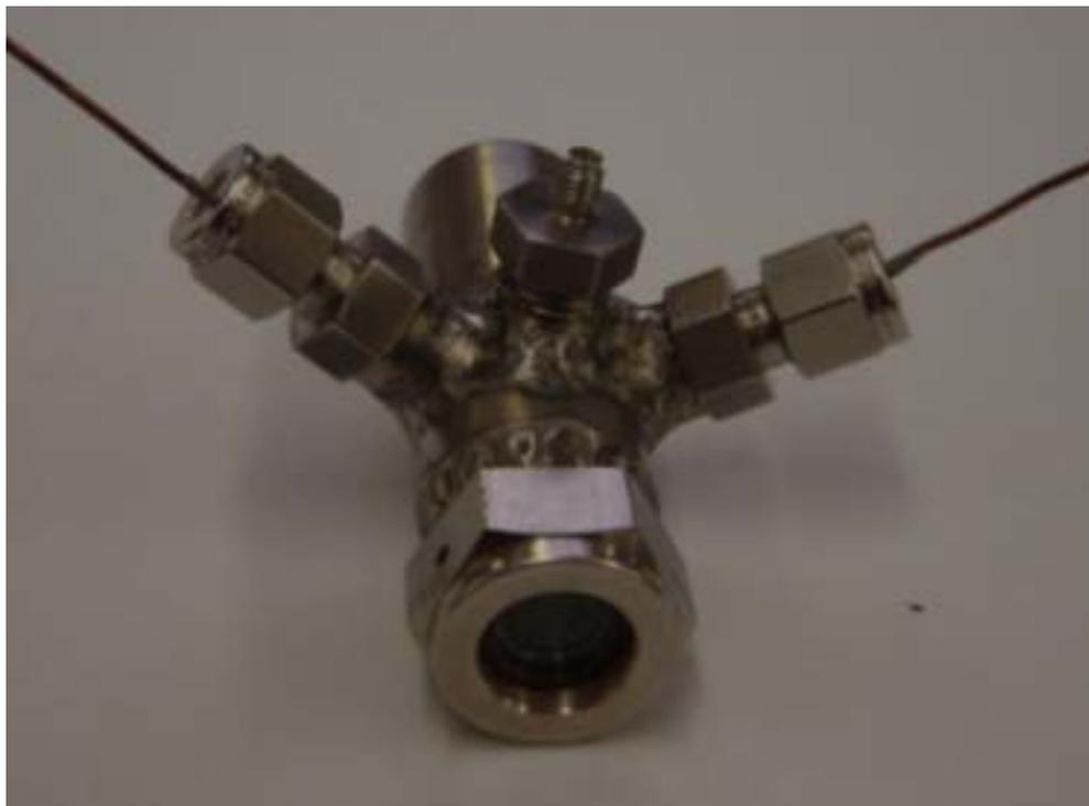
Figure 2.1: The cell is pictured with the capillary on top, electrical feedthroughs to the sides, and the window in front. The rear cap is not pictured. Picture taken from Waegall's MQP thesis [10].
