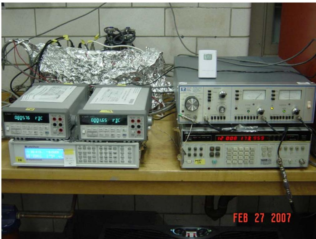
Figure 2.3: Pictured are the electronics used in gathering data. The lock-in amplifier (top right) and function generator (bottom right) are located next to the temperature controller (bottom left) and two agilent multimeteres (top left).
