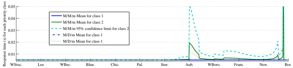
(b) Response time of transmitting packets at an arrival rate of 60 msg/sec and exponential service rate.
