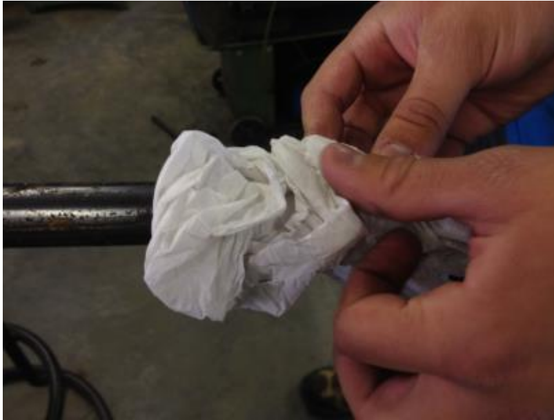
Figure 33: Cleaning pipes with paper towels
