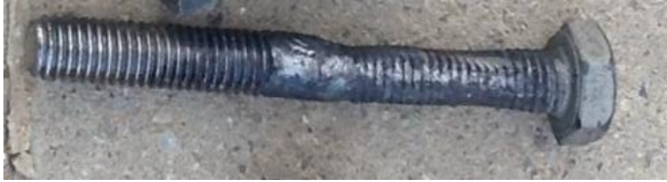
Figure 57: Welded pin made from two bolts
