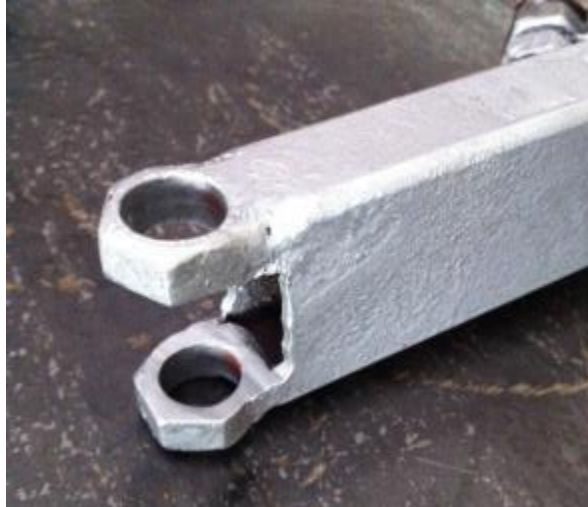
Figure 59: Hex nuts welded to the rectangle
