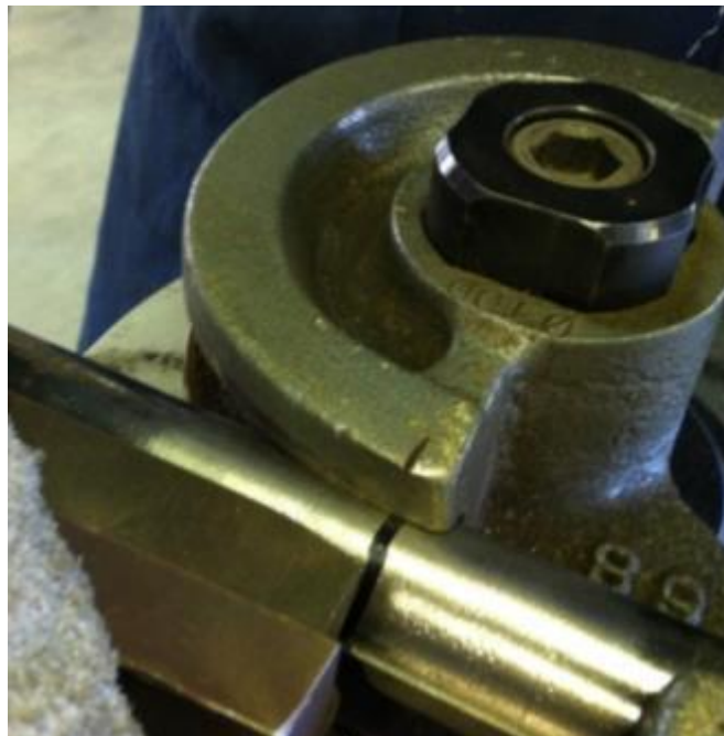
Figure 36: Lining up the pipe with the bender
