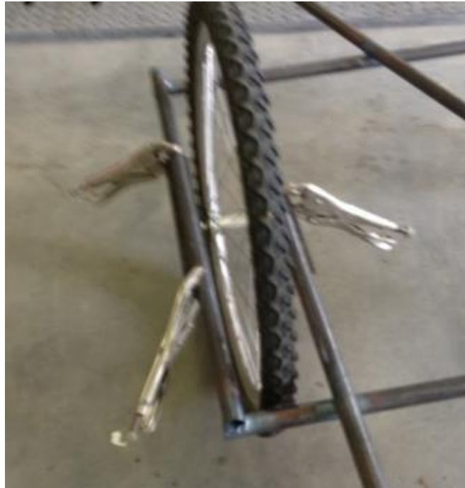
Figure 43: Clamping the wheel angle iron
