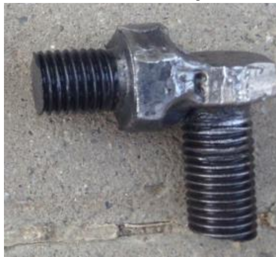
Figure 56: Two #16 bolts welded together
