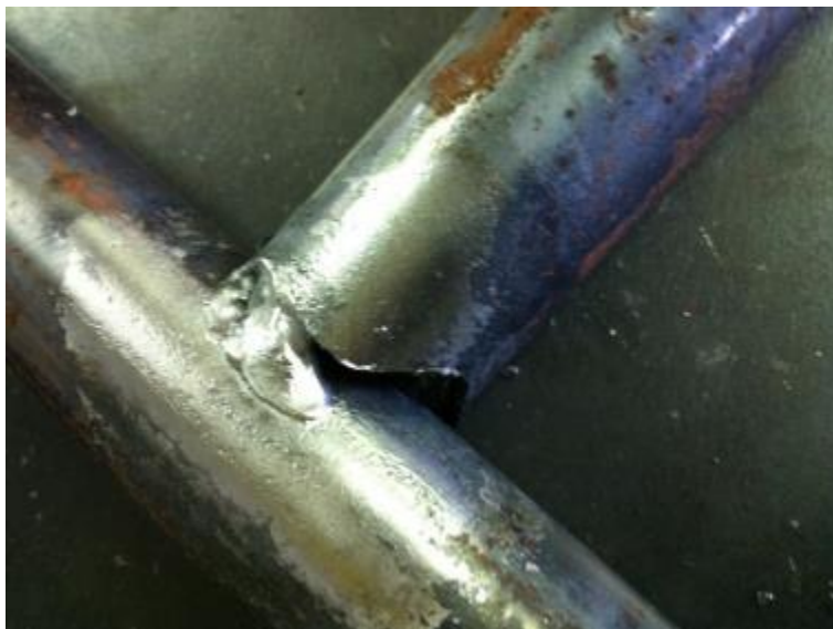
Figure 40: Welding a tack for a joint
