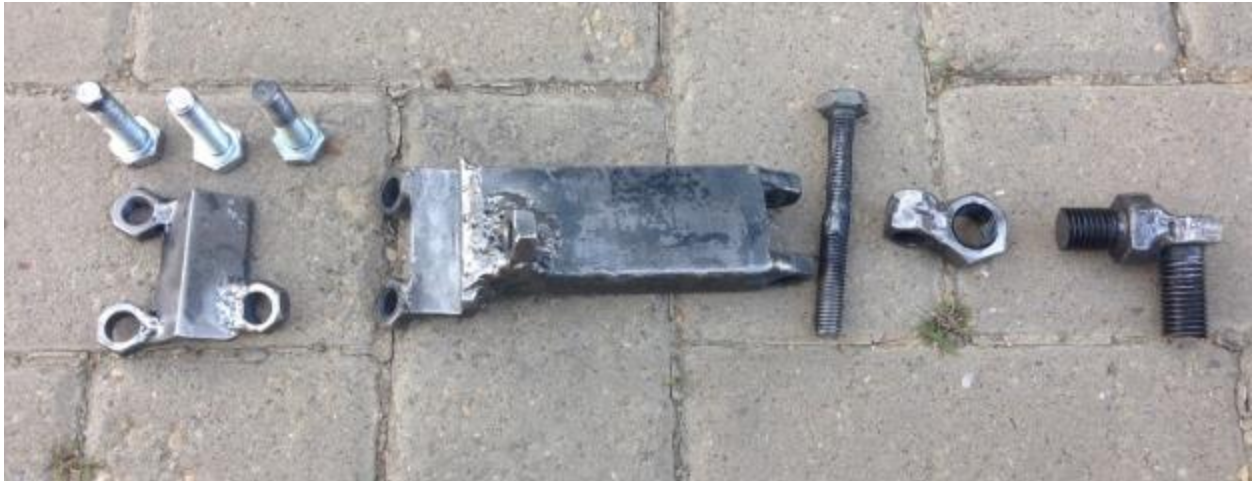
Figure 50: The joint broken down in to its 8 components, left to right, 3-10 mm bolts, clamping plate for seat post, the stock, the pin, welded nut connector, welded bolt connector.
