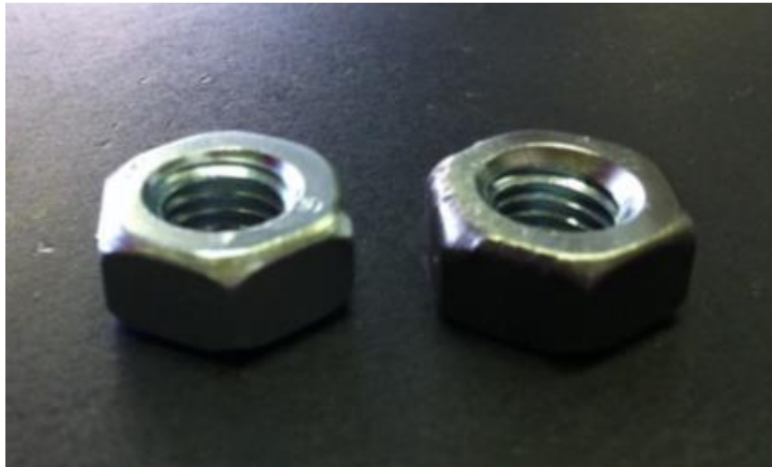
Figure 35: Hex nuts galvanized (left) and de-galvanized (right)
