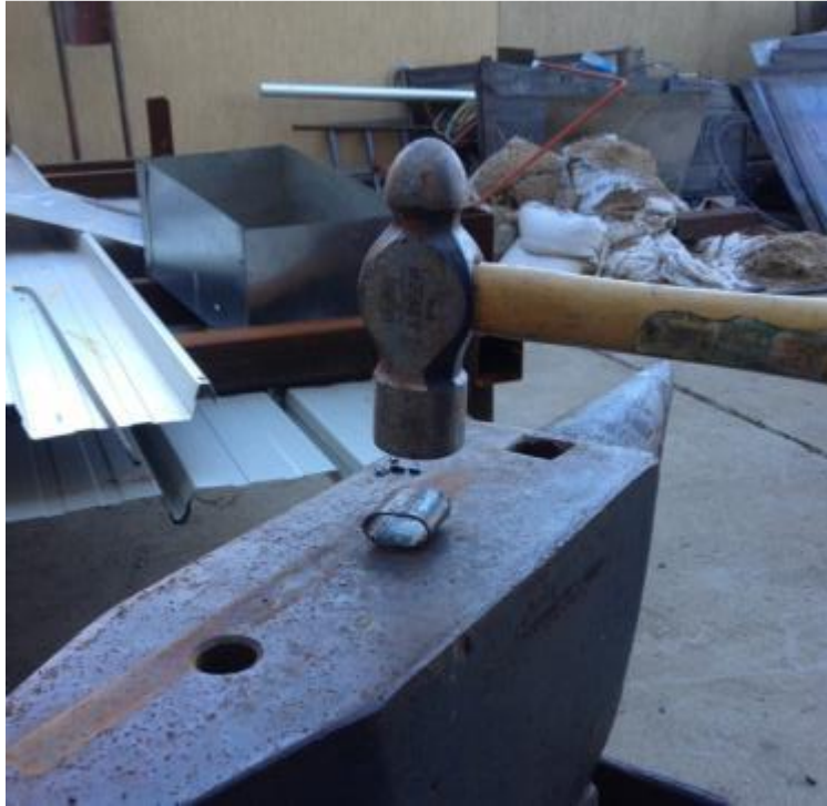
Figure 44: Making a cap with the anvil
