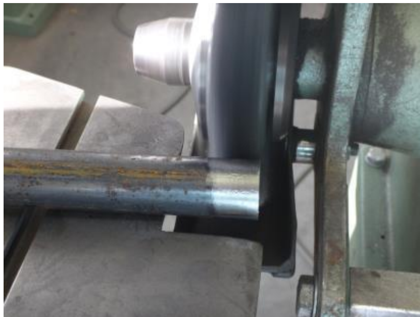
Figure 34: Polishing the steel pipes
