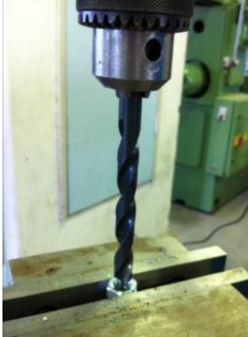
Figure 53: Drilling the threads out of the hex nut
