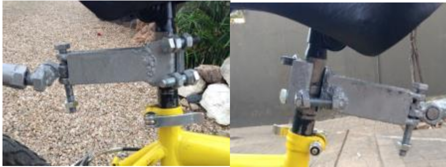
Figure 63: The assembled universal joint painted and connecting the cart to the bicycle
