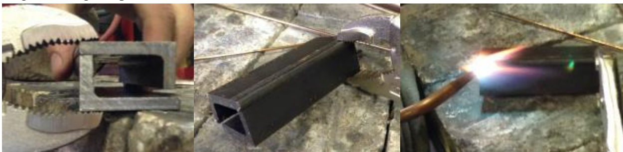
Figure 54: Clamping and welding the rectangle
