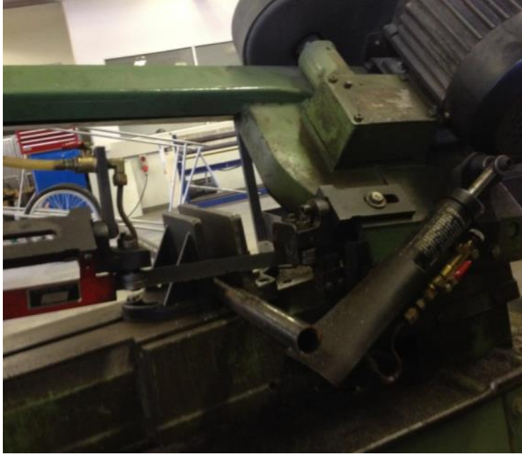
Figure 31: Cutting pipe with a band saw
