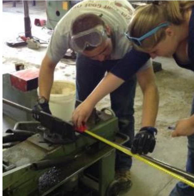
Figure 10: Measuring a pipe for cutting with band saw
