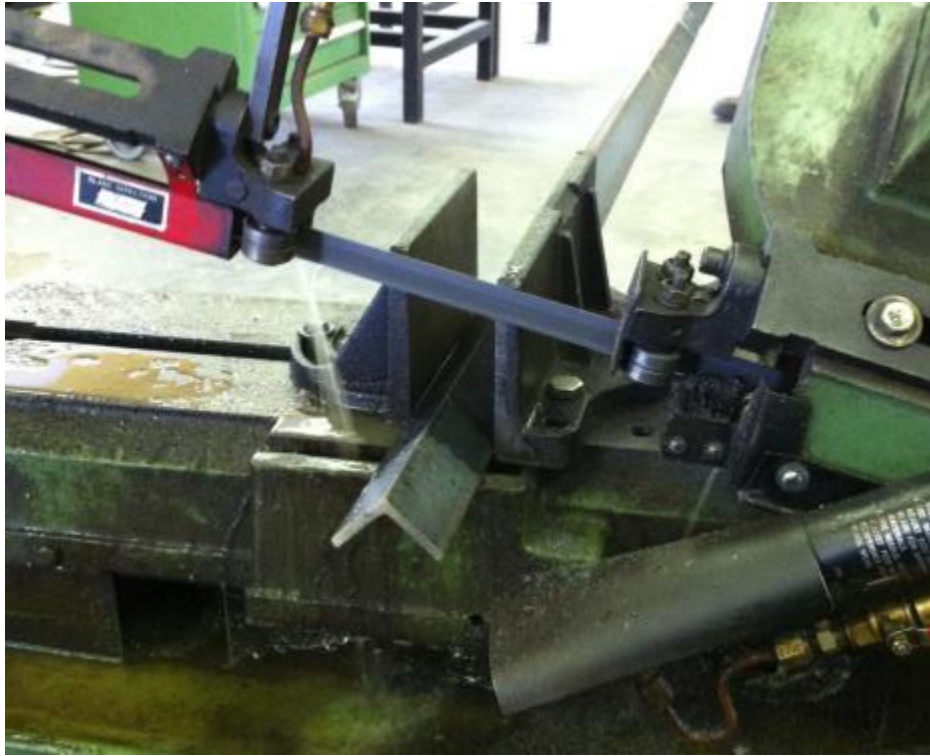
Figure 32: Cutting angle iron with a band saw
