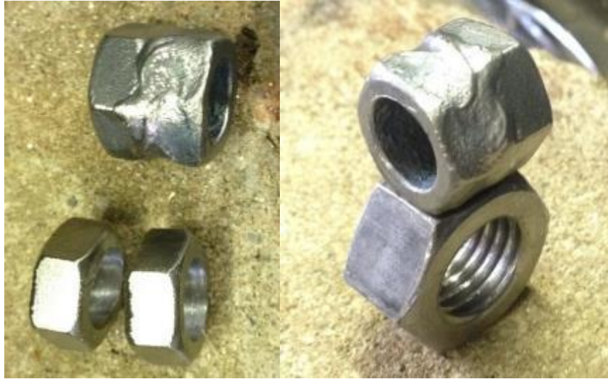
Figure 55: Welding together three hex nuts
