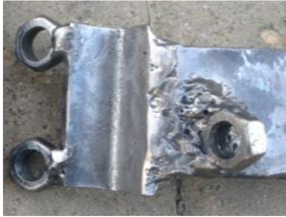
Figure 61: Lining up the third hex nut
