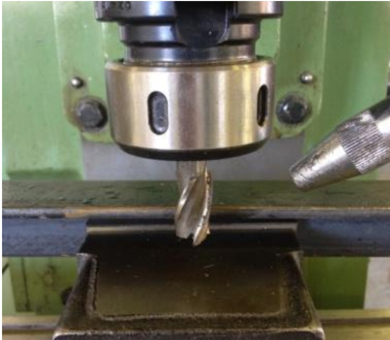
Figure 39: Milling the wheel channels
