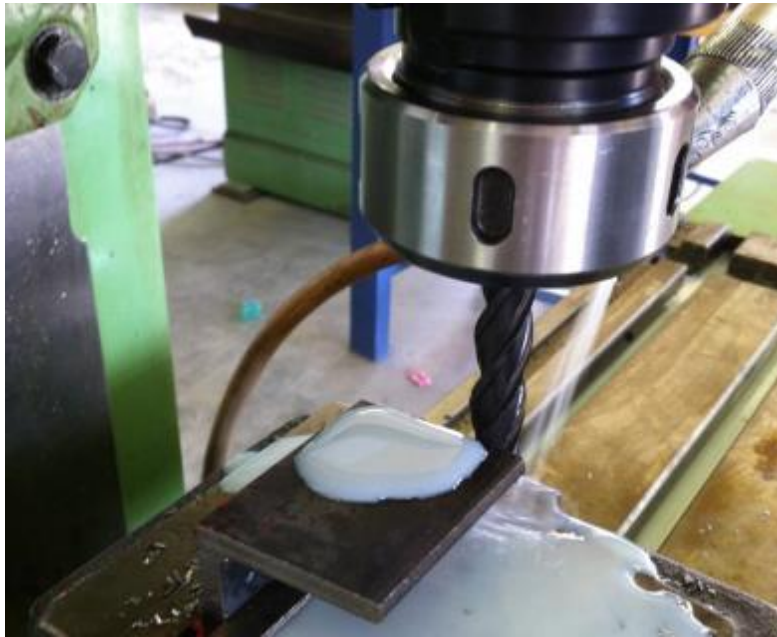
Figure 51: Milling the angle iron
