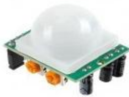
Figure 32: Arduino PIR motion sensor component
