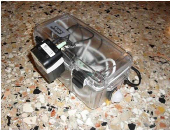
Figure 31: Installation inside OtterBox
