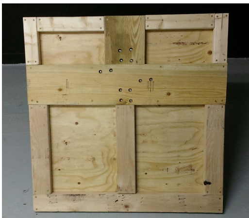
Figure 40: Bottom of the Winching Platform
