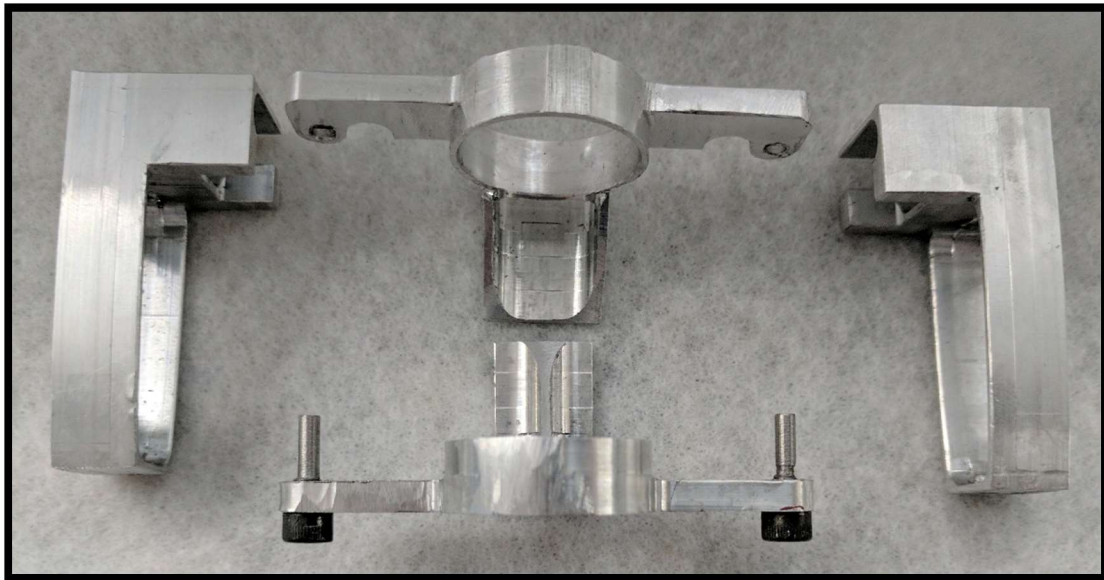
FIGURE 36: FINISHED BUT UN-ASSEMBLED ALUMINUM TAIL JOINT PIECES
