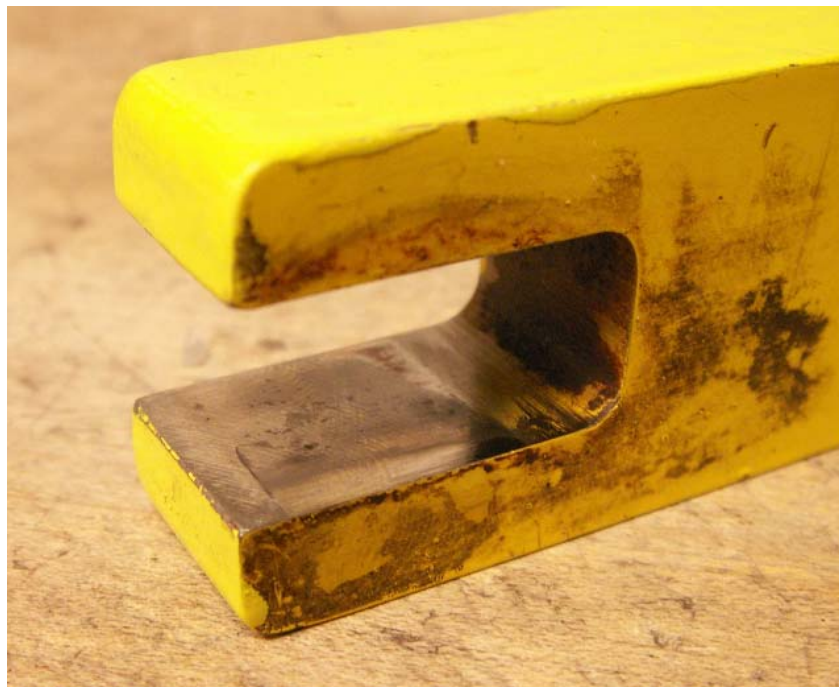
Figure 23: Stripper Tooling Lever Wear
