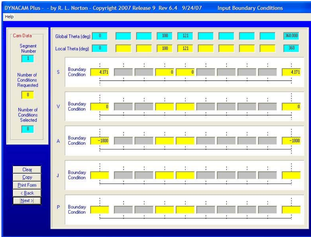
Figure 33: Boundary Conditions for Redesigned Stripper Cam
