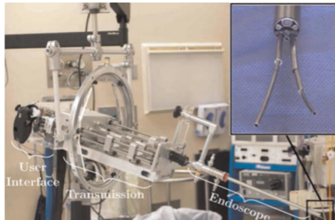
Figure 2.7: Hand-held robot for transurethral laser surgeries with (top right) a close-up of the endoscope with 2 of the manipulators. Reproduced from [6].
