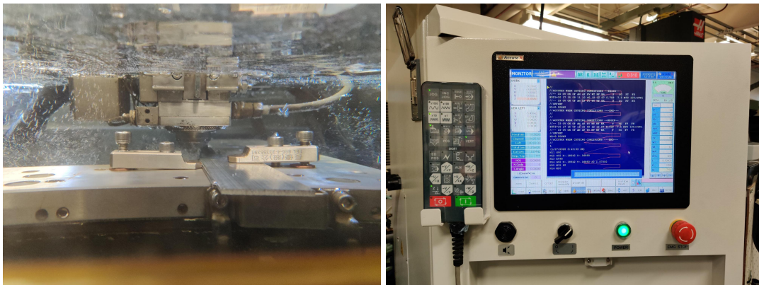
Figure 2.5: Wire EDM machining setup. Left: Nitinol tube fixture during cutting. Right: G-code display and cutting parameters.
