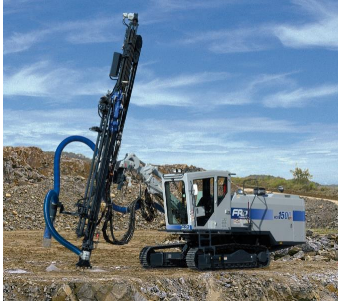
Figure 27: Downhole Drill Example from “Blast Hole Drills.” Furukawa Rock Drills | Furukawa Rock Drill Parts, www.canyonequipment.com/mobile/subcategory/rock-drilling/blast-hole-drills .
