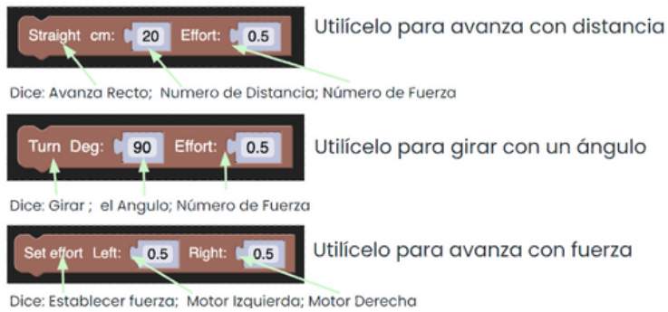
Figure 25: An example of the reference sheet explaining some of the blocks of code.
