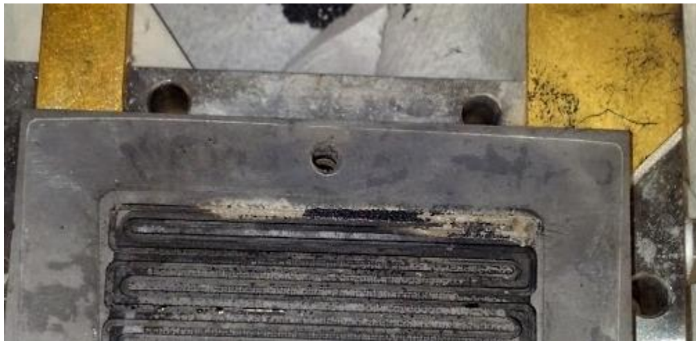
FIGURE 22: RESIDUE FOUND TO BE BLOCKING THE GAS INLET TO THE CELL (UPPER RIGHT OF SERPENTINE CHANNEL CONFIGURATION)
