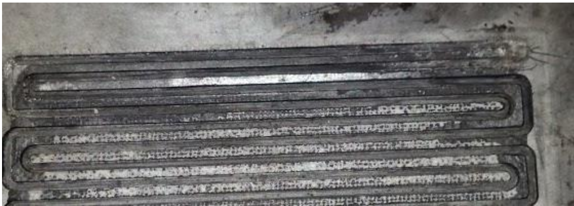
FIGURE 25: BLOCKED SERPANTINE CHANNELS IN THE GRAPHITE PLATE
