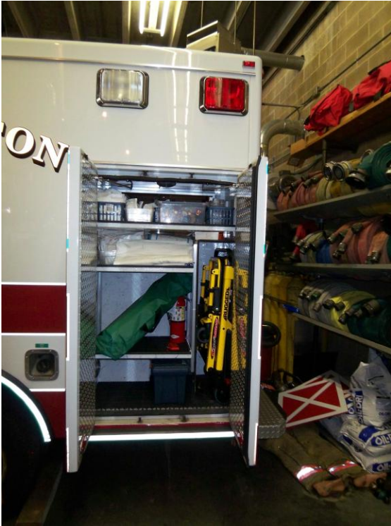
Figure 12: Storage of stairchair and tools
