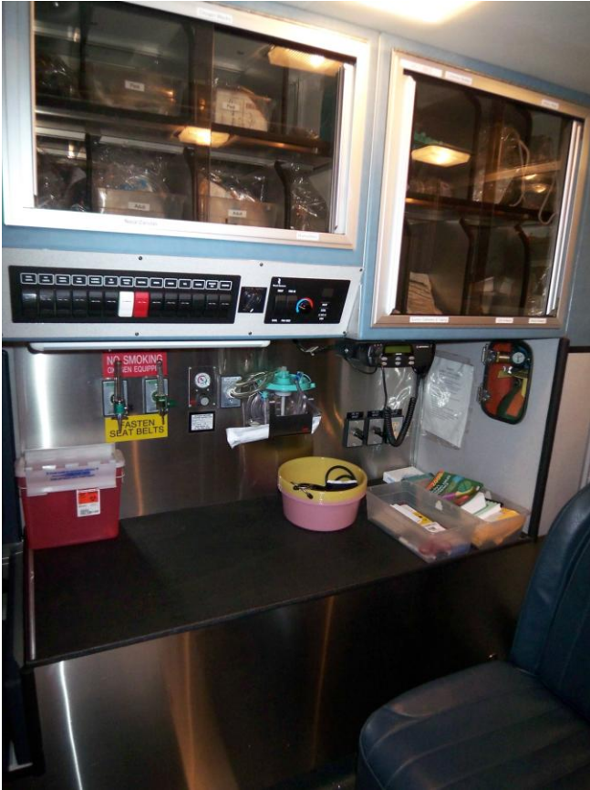
Figure 9: Storage of various medical supplies and fluid and oxygen controls
