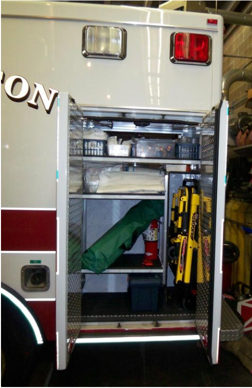
Figure 20: External storage of stairchair and tools
