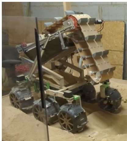
(NASA Lunabotics 2022 Pol | Atlas | University of Illinois at Chicago, 2022) Figure 6: UIC's entry from last year whose conveyor is angled at 90 degrees to bring regolith into their bucket. Their filter was not the best though.
