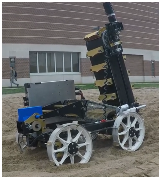
(Purdue Lunabotics Proof of Life Submission 2022, 2022) Figure 5: Purdue's entry from last year which uses a mesh attached to some frame members as a filter
