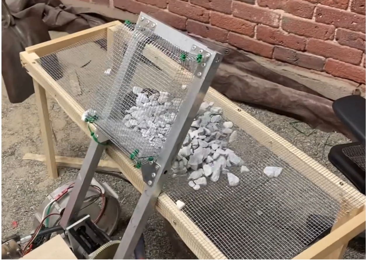
Figure 46: The bucket depositing gravel on the center of the sieve
