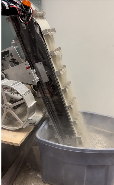
Figure 43: Testing the excavator digging down to depths where gravel would have been encountered
