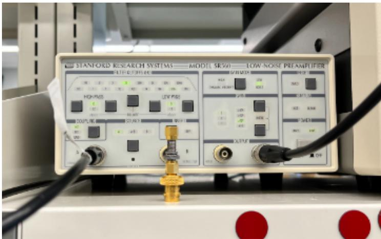
Figure 16: The pre-amplifier that minimizes the noise to produce a cleaner signal.
