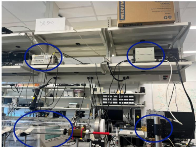
Figure 12: The output and reference part of the spectrometer. Circled from top left to bottom right: the wave generator, the power supply/multiplier, the signal generator, and the output.
