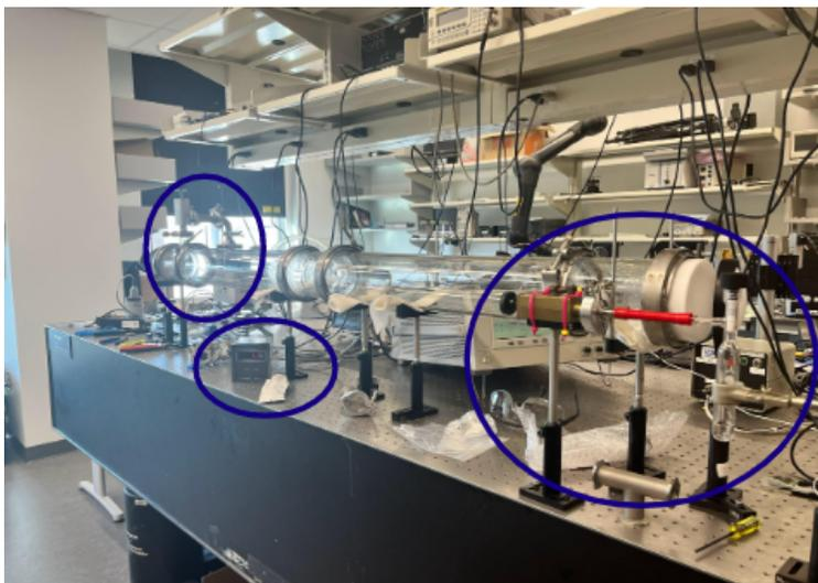
Figure 13: The cell of the spectrometer with the three subsections, seen in blue circles. From left to right, are the diffusion pump, the pressure gauge, and the sample.
