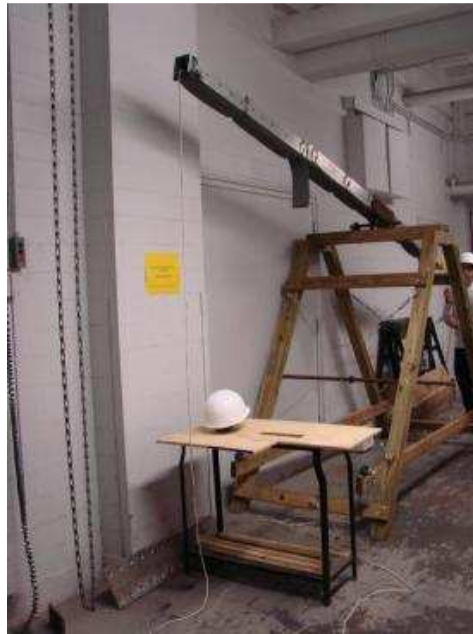
Figure 26: Setup of Cantaloupe Test
