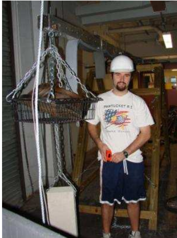
Figure 30: The Beam Weighted Down
