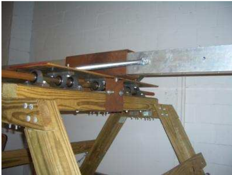
Figure 24: Lock Out Mechanism in Place
