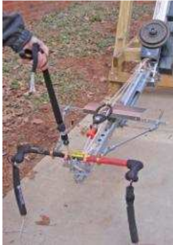
Figure 14: Kite Control Mechanism Attached to Rocking Arm
