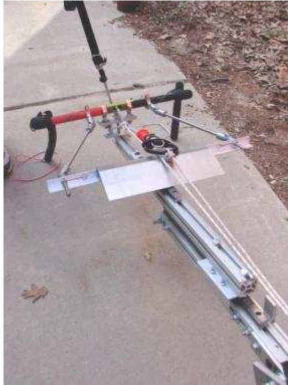
Figure 13: New Kite Control Mechanism as Built
