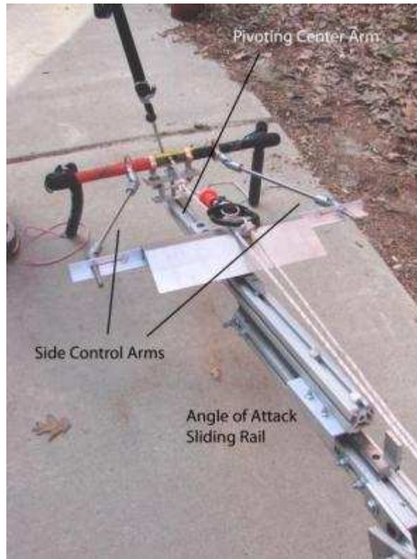
Figure 9: Kite Control Mechanism
