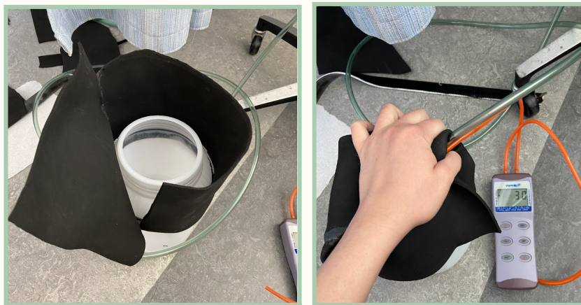
Figure 44: Plastic Cylinder Container with Velcro Sealing Test.
