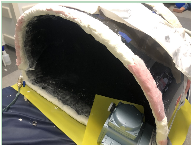
Figure 60: Proto-putty Encasing Edges of Neoprene.
