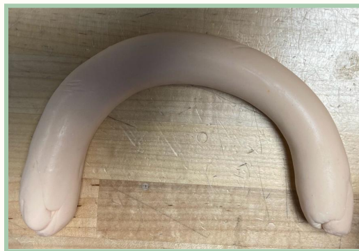
Figure 46: Combination of Silicone Caulk and Cornstarch.
