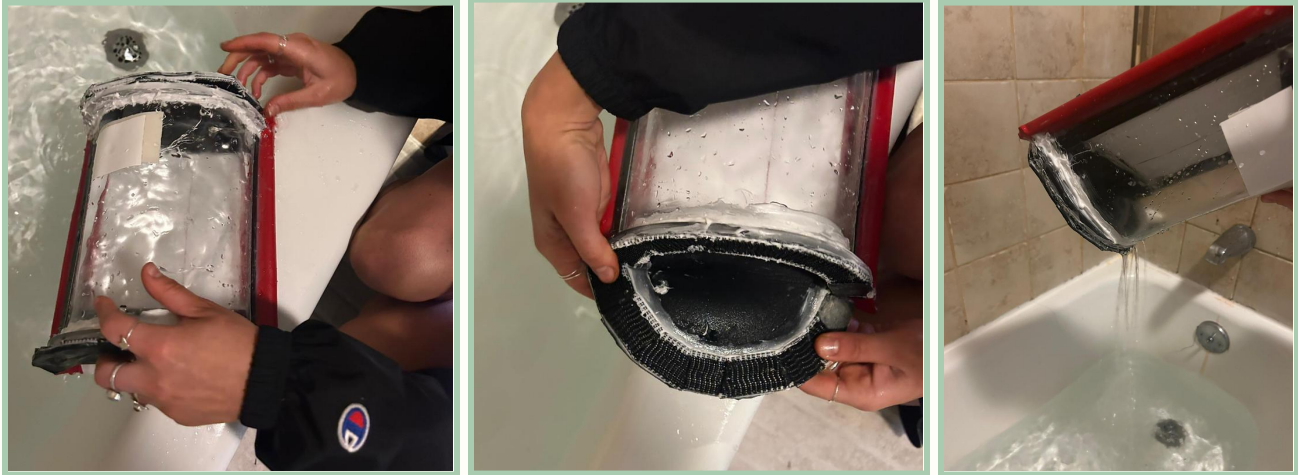
Figure 45: Water Submersion Test Using Small-Scale Prototype.
