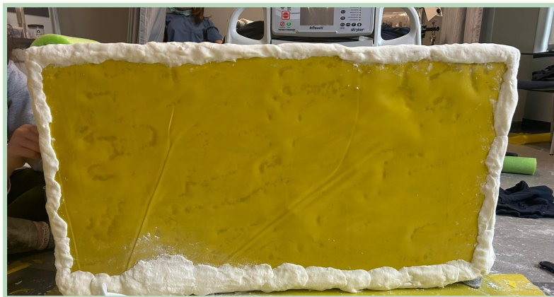
Figure 62: Plastic Sheet Covering Wooden Frame.
