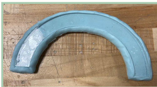
Figure 47: Silicone Rubber Molded to Acrylic Gasket Part.
