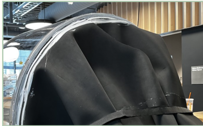
Figure 55: Neoprene Connected to the Shell Through Velcro on the Inside of the Shell.
