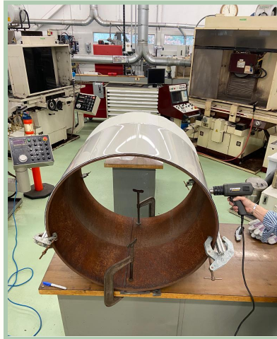
Figure 37: First Attempt to Mold Polycarbonate Sheet.
