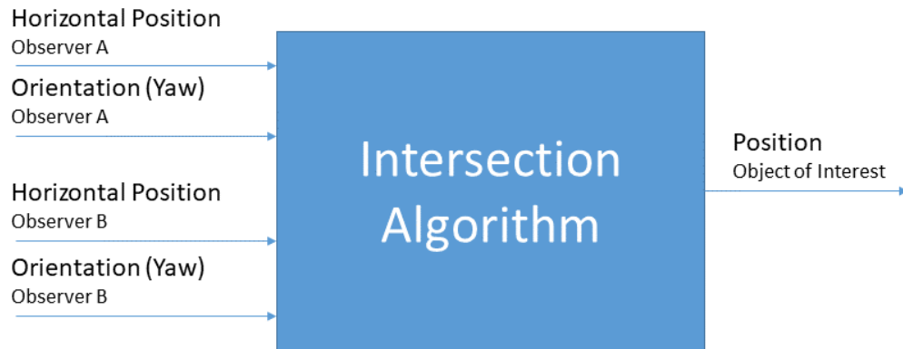
Figure 4-14: Two-Dimensional Intersection Algorithm System Block
