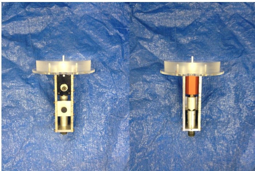
Figure 43: Torque-Monitoring Device Front and Back
