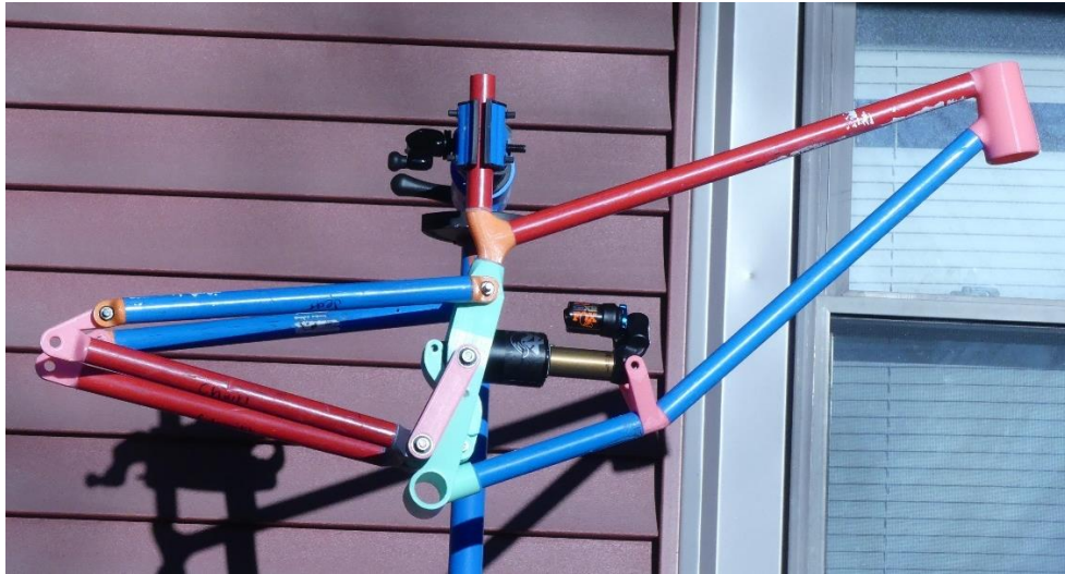
Figure 16: The fully assembled 3D printed prototype
