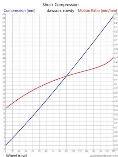
Figure 7: graph showing the shock compression and motion ratio
