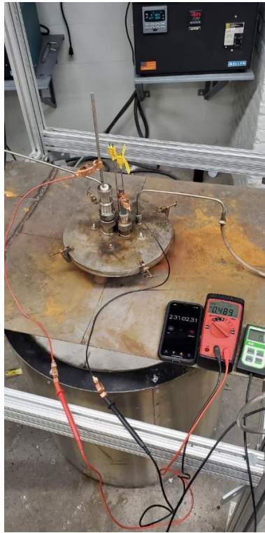
Figure 37: Maximum voltage of 0.489 V obtained using alloy 2 (37.5 Fe – 30 Mn – 30 Sn – 2.5 C).
