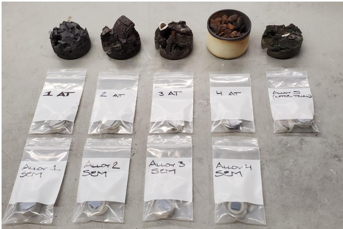
Figure 35: Condition of alloys after OCV experiments.
