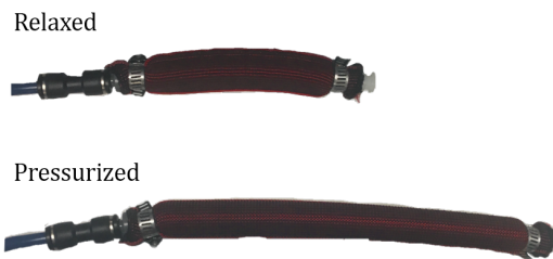
Figure 2.1: Expansion and contraction of Hydro Muscle (Sridar et. al., 2016)
