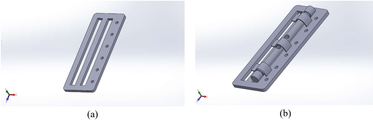
Figure 18(a-b): (a) Two-Slotted Buckle with Six Extruded Holes. (b) Two-Slotted Buckle with Six Extruded Holes and Hooks for Rod.
