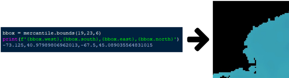
Figure 6: Demonstrating a conversion from Spherical Mercator Conversion to latitude longitude bounding box. This was an important step for being able to quickly generate tiles for testing.
