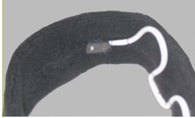
Figure 4.6. Elastic headband used for sensor attachment to the forehead.
