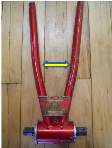
Figure 9: Bottom bracket with attached seat stays.
