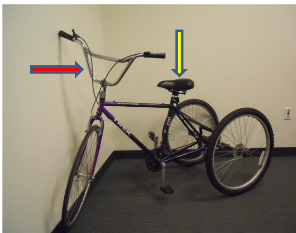
Figure 13: The handlebars (red) and wide seat (yellow) promote an upright and supported seating position.
