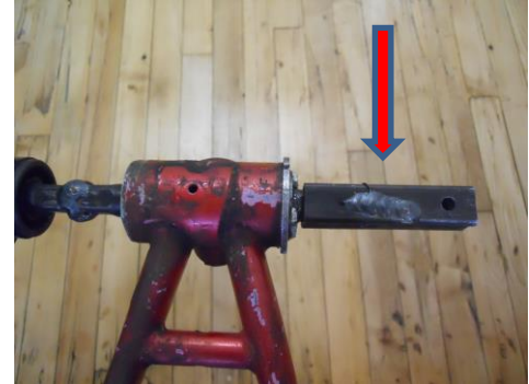
Figure 10: Square stock steel sleeve welded onto bottom bracket axle.
