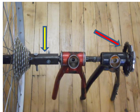
Figure 15: Shows connection between the drive wheel and the drive side of the axle (yellow), with single gear (red).
