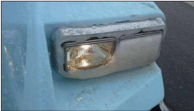
Figure 2 – Snow accumulation on LED Headlight [12]
