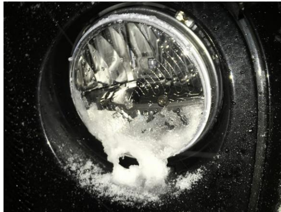
Figure 4 – Snow Accumulation on Jeep Headlight [14]
