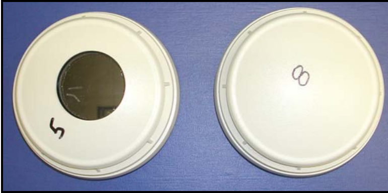
Figure 9 -- Photoelectric smoke detectors with (l), and without (r) optical access.
