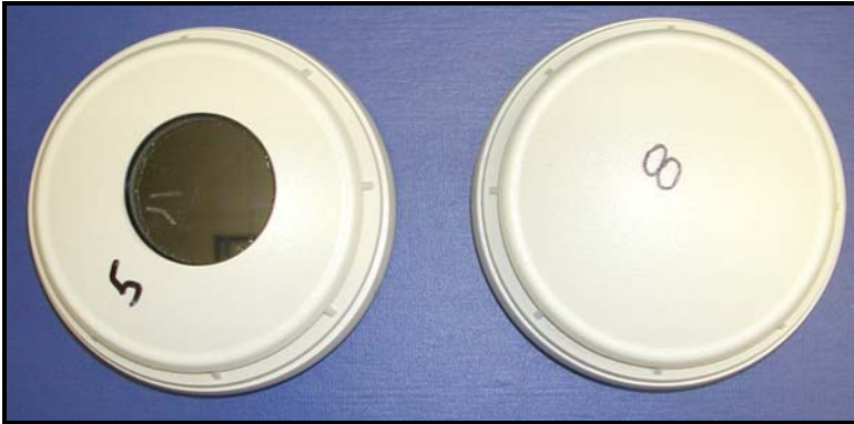
Figure 15 -- Photoelectric smoke detectors with (l), and without (r) optical access.
