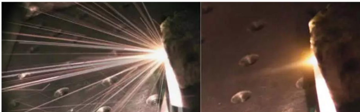
LASER BEES: ZAPPING OLIVINE ROCK WITH A LASER Laser Bees asteroid deflection project: zapping olivine rock with a laser, this shows the ablation response of the olivine on the left, with ejecta (pieces) coming out, and on the right with a mini "rocket plume".
