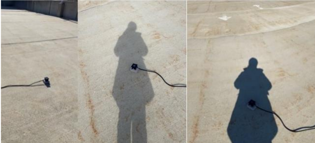
Figure 13: Light sensors outdoors, exposed to partly cloudy suns around midday. Going from left to right is no shadow cast, slight shadow cast, and dark shadow cast
