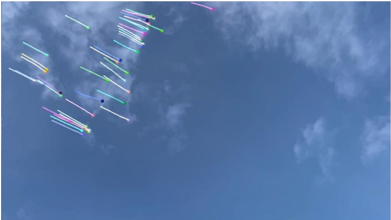
Figure 20: Lines showing clouds movement tracked with sparse optical flow
