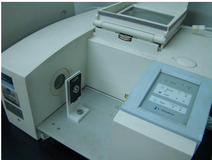
Figure 29. FTIR spectroscopy setup (light beam pass through the circular hole on the spectrum sample holder).
