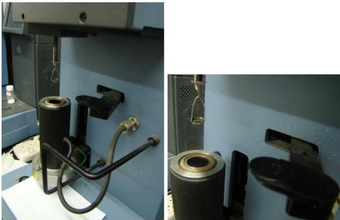
Figure 31. Sample contained in the Platinum pan being loaded into the electrically heated oven.
