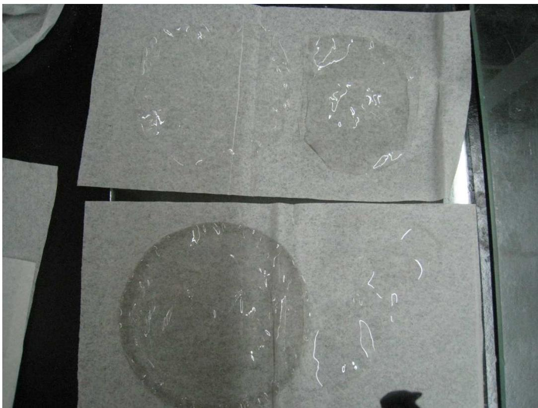
Figure 37. Fabricated membranes – upper left: 0.1 wt% CNT-PVA/Nafion; upper right: recast Nafion; lower left: 0.05 wt% CNT-PVA/Nafion; lower right: commercial Nafion<sup>®</sup> 212.
