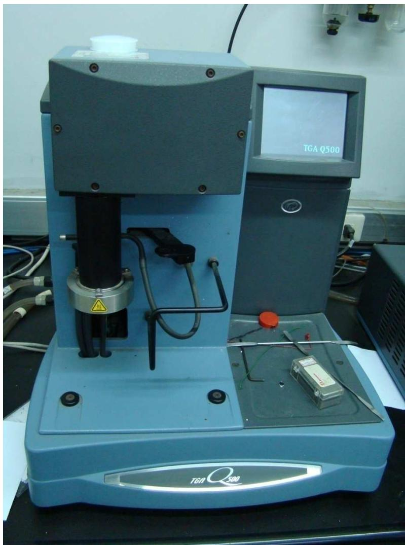
Figure 30. Thermogravimetric Analysis Instrument TGA Q500.
