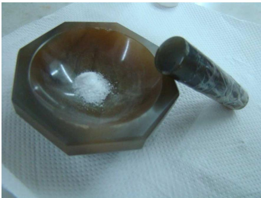
Figure 25. Finely grounded mixture of CNT-PVA and KBr in a mortar.
