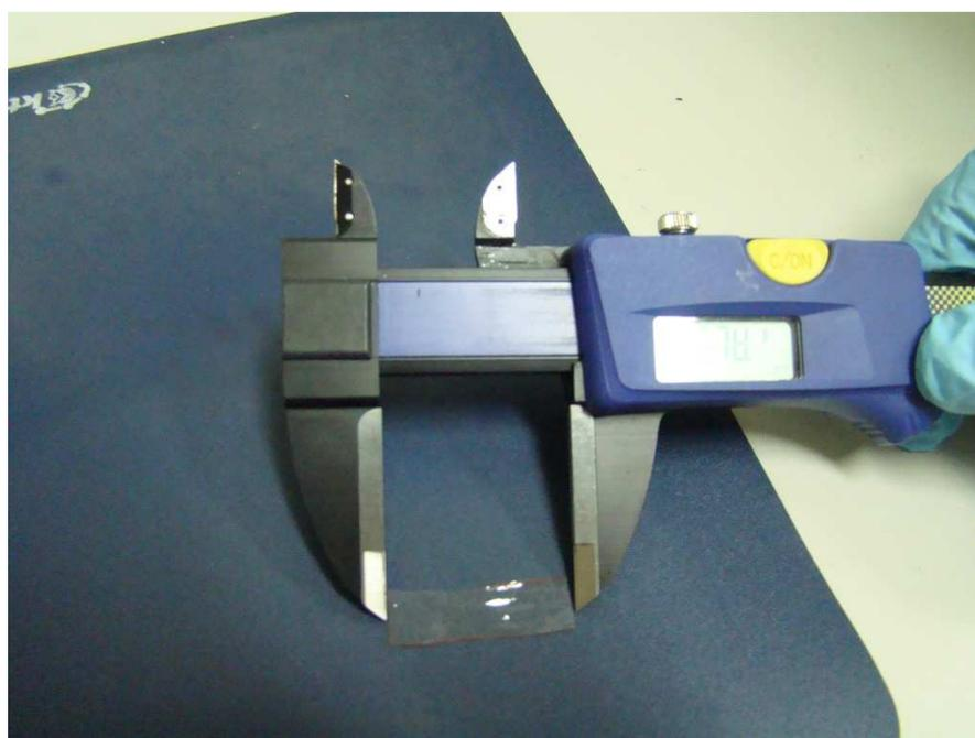
Figure 40. Measuring the length of membrane between two Instron clamps.
