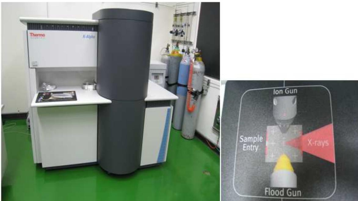
Figure 32. XPS machine and its three guns.
