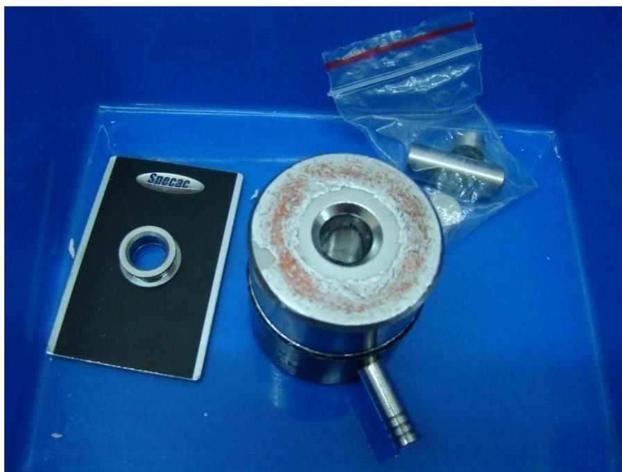
Figure 26. Special die (on the right) and spectrum sample holder (on the left).
