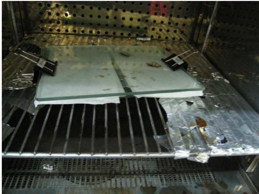
Figure 36. Acidified membranes put in drying oven overnight.
