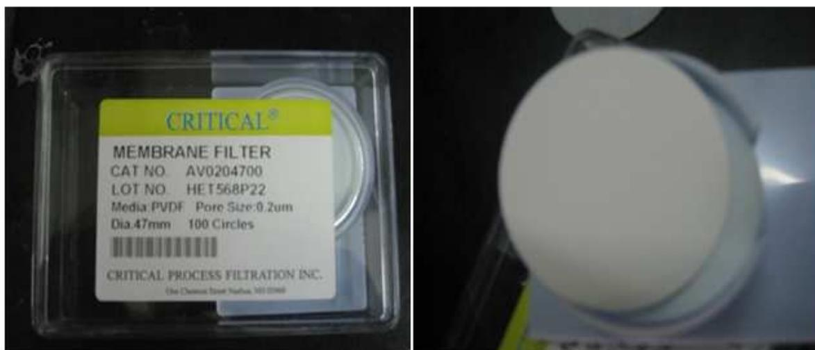
Figure 22. Membrane filter box (on the left) and membrane close-up view (on the right).
