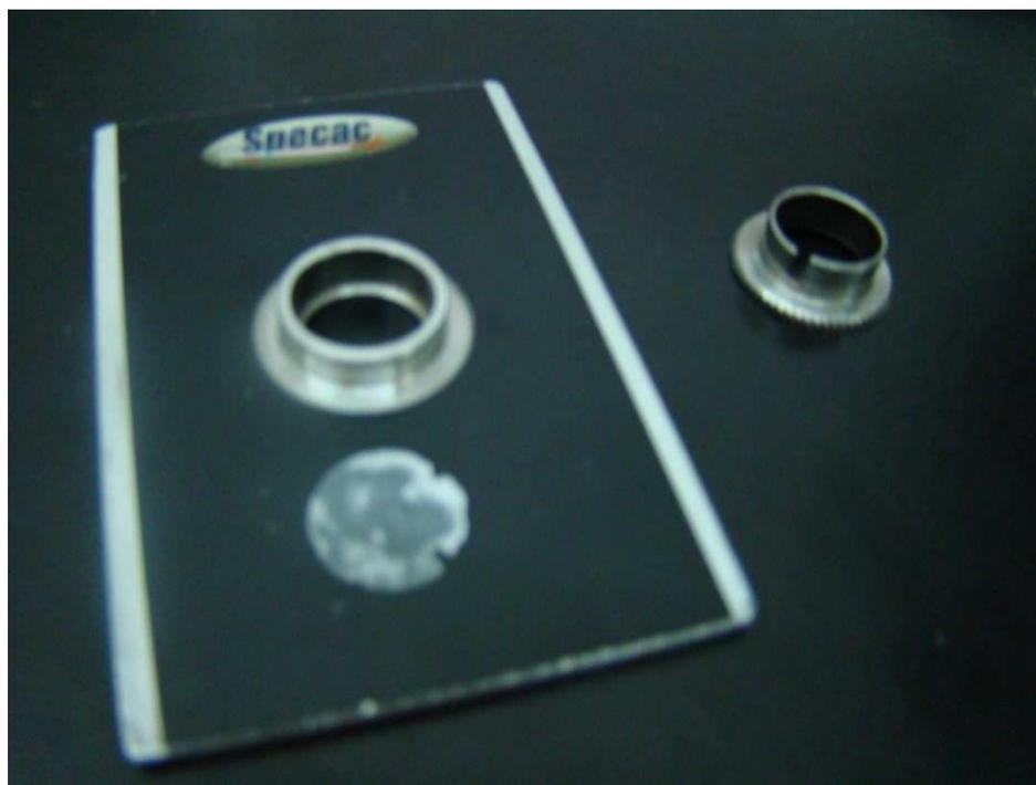
Figure 28. A transparent disk of CNT-PVA/KBr on Specac.
