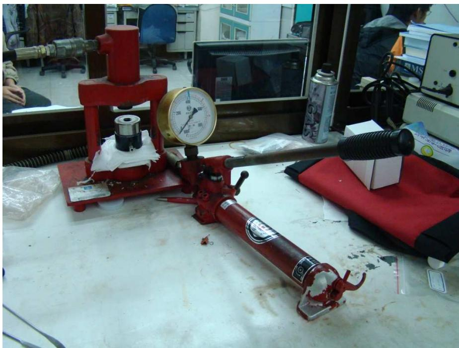
Figure 27. Standard press with capacity of 1000 kg-f/cm<sup>2</sup>.
