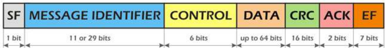
Figure 10 CAN bus message structure [2]
