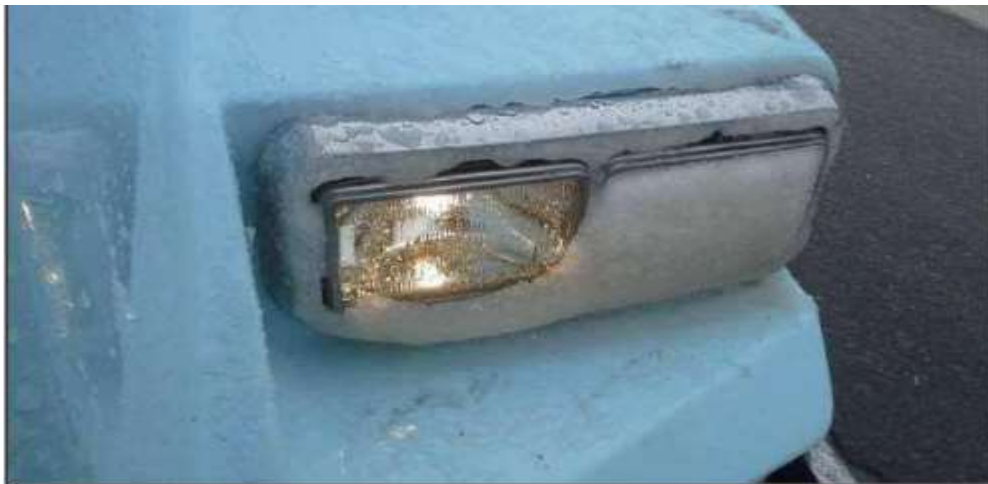
Figure 8 Snow accumulation on LED headlight [1]
