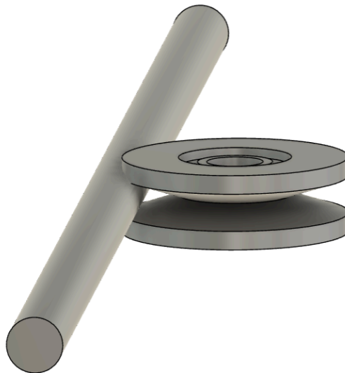
Figure 90: Single Rod-Single V-Groove Bearing Travel Interface
