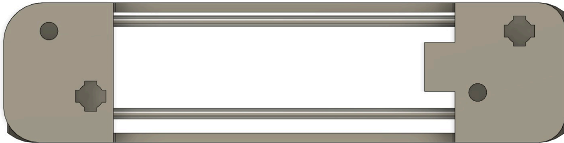
Figure 89: Linear Rods after Full Insertion (Top View)
