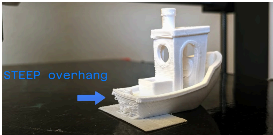
Figure 27: Front Overhang Caused by the Angled Extruder of a Belt Printer (O'Connell, 2023)
