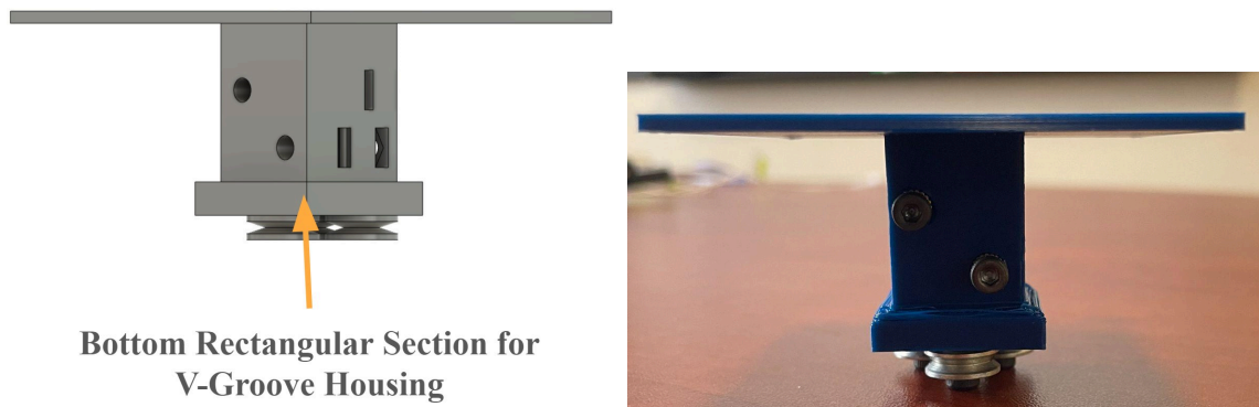
Figure 87: Bottom Rectangular Section for V-Groove Bearing Housing (Left: CAD, Right: Physical)
