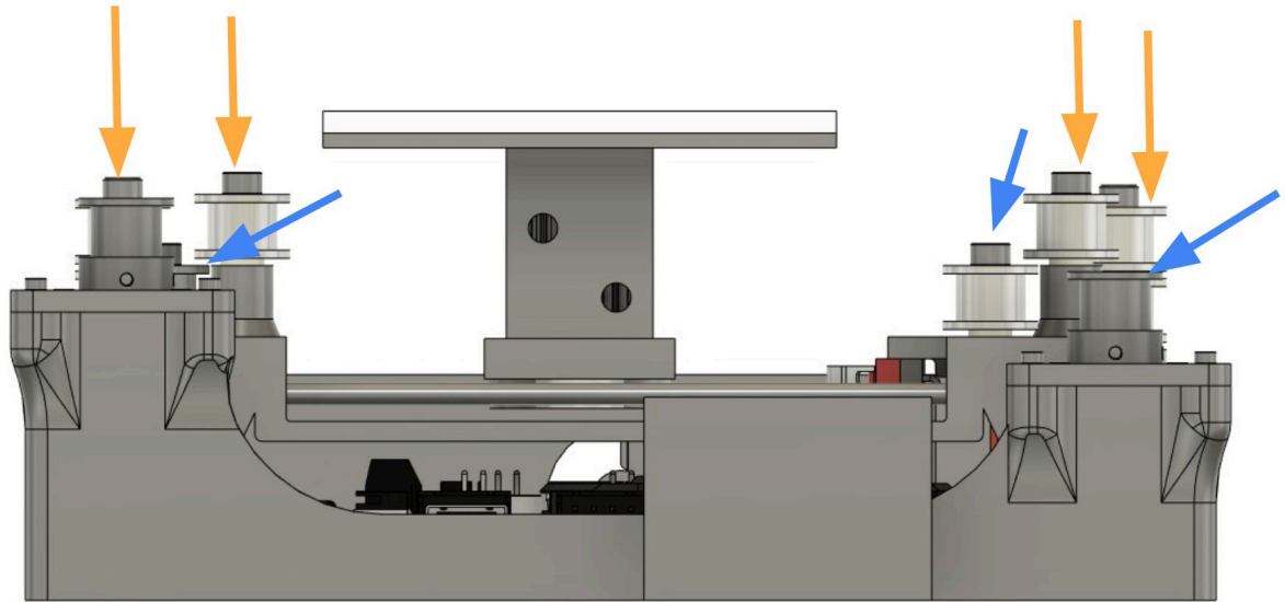
Figure 100: Overall V-Groove Pulley Alignment between the Gantry and Bed Holder Movements
