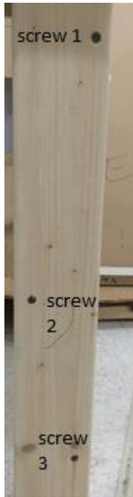
Figure 18: Screw placement for table leg
