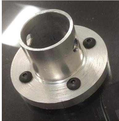
*Figure 29: Shaft attachment collar*
