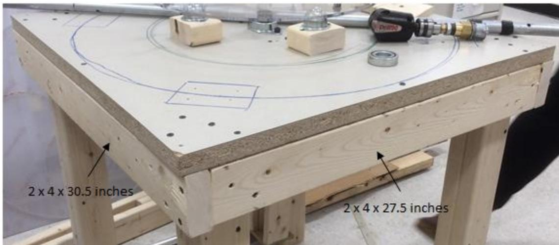
Figure 19: Supporting frame of table
