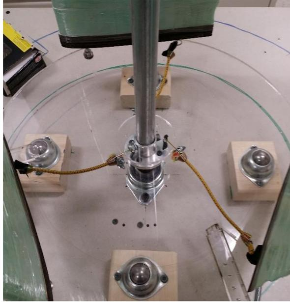
*Figure 13: Articulating airfoil design using bungee cords*
