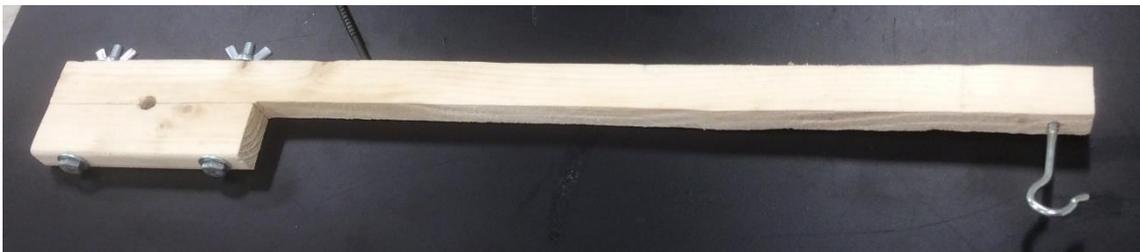
*Figure 24: Constructed prony brake*
