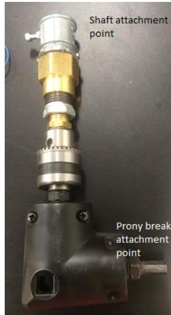
*Figure 23: 90 degree angle motion adjustment*
