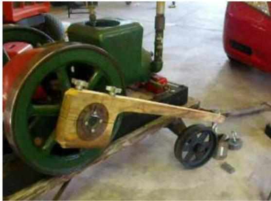
*Figure 22: Example prony brake*
