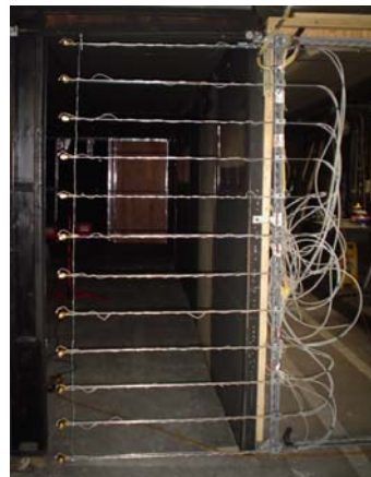
Doorway with movable array of bi-directional probes and thermocouples
