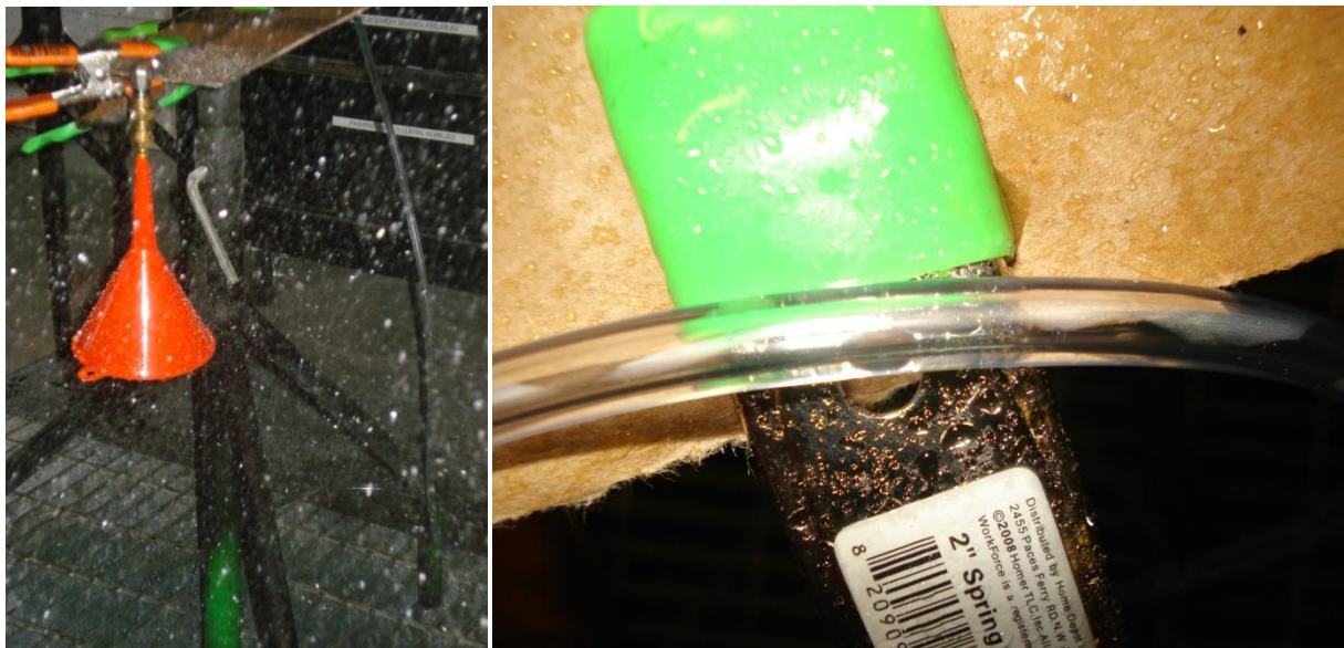
Figure 6: Left: Test setup of prototype showing probe in water spray. Right: Results from Run 4 showing no water in tubing.
