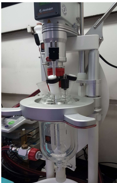
Figure 10 The Experimental Setup of the 500mL Thermocouple experiments
