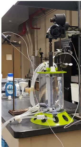
Figure 11 The experimental setup for the 3L thermocouple experiment
