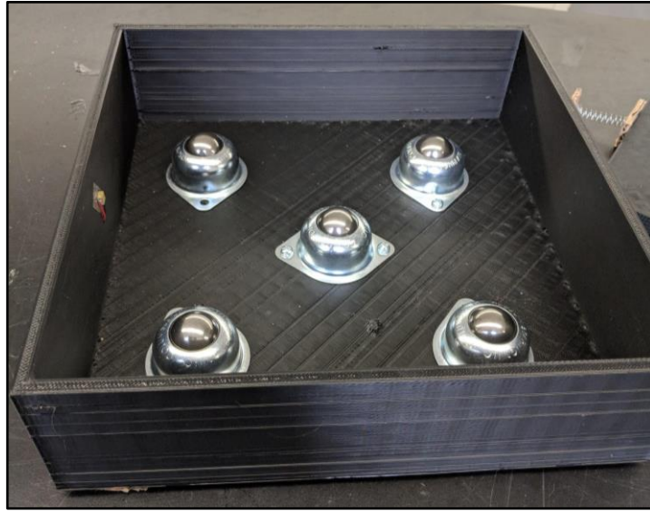
Figure 15: Base box with Ball Bearing Transfer Units
