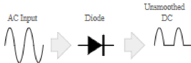
Figure 4: Signal Response from a Diode [38]
