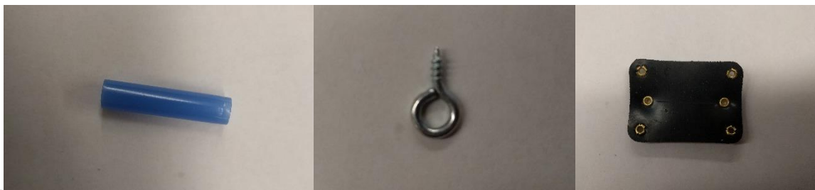
Figure 14: Various tested tendon sheathing methods, from left to right: straws, eye screws, 1/16 inch EPDM with grommets thread holes
