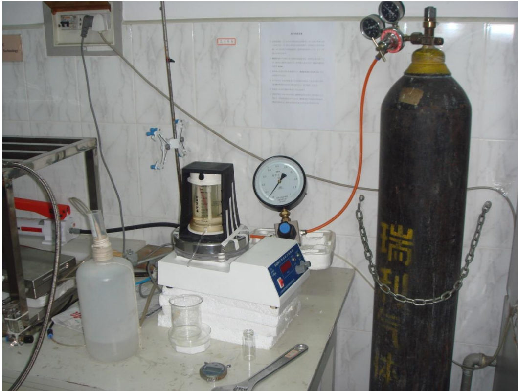
Figure 6 Picture of the ultra-filtration unit
